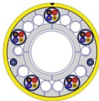
Fig. 7.4 Control Umbilical Picture
